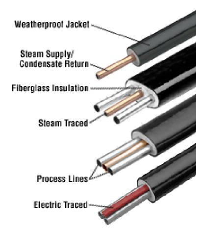
A tubing bundle is a small diameter tube or group of tubes packaged in an insulated, weatherproofed jacket. It's either steam or electric traced to provide freeze protection or temperature maintenance of process fluid or gasses.
