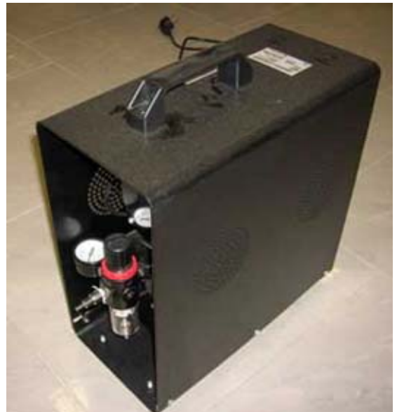
Figure 2-6. Service Air Compressor
