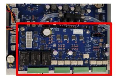
i. For removing the relay board, note the position of the four screws securing the relay board to the mainboard, as shown below, and remove any connections that may be installed on the board at this time.
