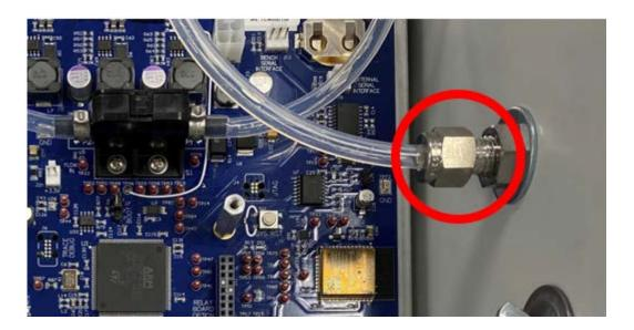
5. Next, loosen the tubing nut from the exhaust port of the analyzer (shown below) by using the same method and wrenches previously listed in step 4.
