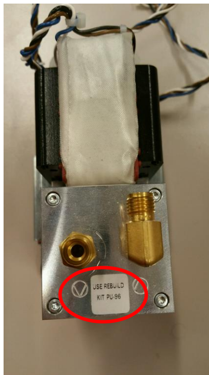
Location of rebuild sticker (Top View)
