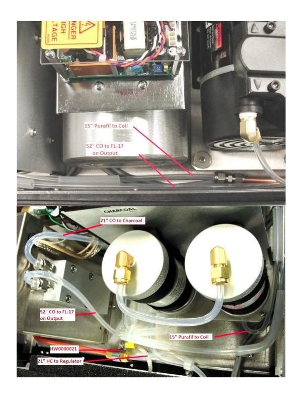
INSTALLING HC/CO SCRUBBER IN 701 GEN-4 NOTE15-02 Rev A (7121) Approval date here Page 6 of 6 PRINTED DOCUMENTS ARE UNCONTROLLED
