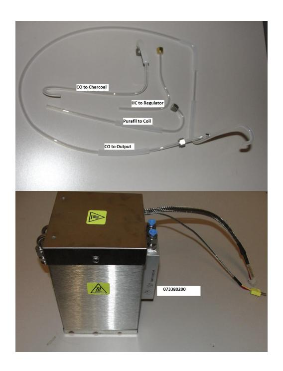
INSTALLING HC/CO SCRUBBER IN 701 GEN-4 NOTE15-02 Rev A (7121) Approval date here Page 3 of 6 PRINTED DOCUMENTS ARE UNCONTROLLED
