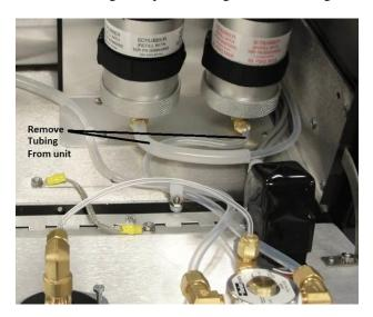
2: install HC/CO scrubber with 4 SN0000228 screws from bottom of instrument.
