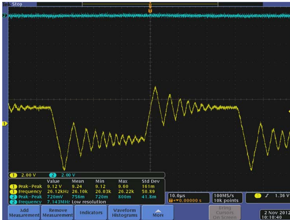
Figure 11 Unadjusted Capacitor Waveform with LED Unplugged
