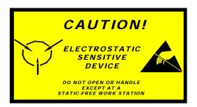
The electronics used in T-API analyzers are sensitive to Electrostatic Discharge (ESD). When working on any T-API device, please ensure that you are properly grounded prior to handling or touching any electronic circuitry in the analyzers! For more information on how to protect sensitive components from ESD during handling, please contact T-API customer service and ask for the ESD Service note number 03-022A.
