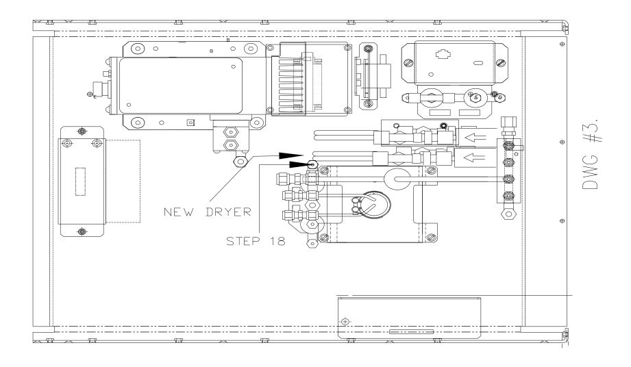
Retrofit of Dryer for Sample and IZS in M200E Analyzer 04-009 Rev C Page 6 of 7
