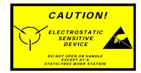
The electronics used in T-API analyzers are sensitive to Electrostatic Discharge (ESD). When working on any T-API device, please ensure that you are properly grounded prior to handling or touching any electronic circuitry in the analyzers! For more information on how to protect sensitive components from ESD during handling, please contact T-API customer service and ask for the ESD Service note number 03-022A.
