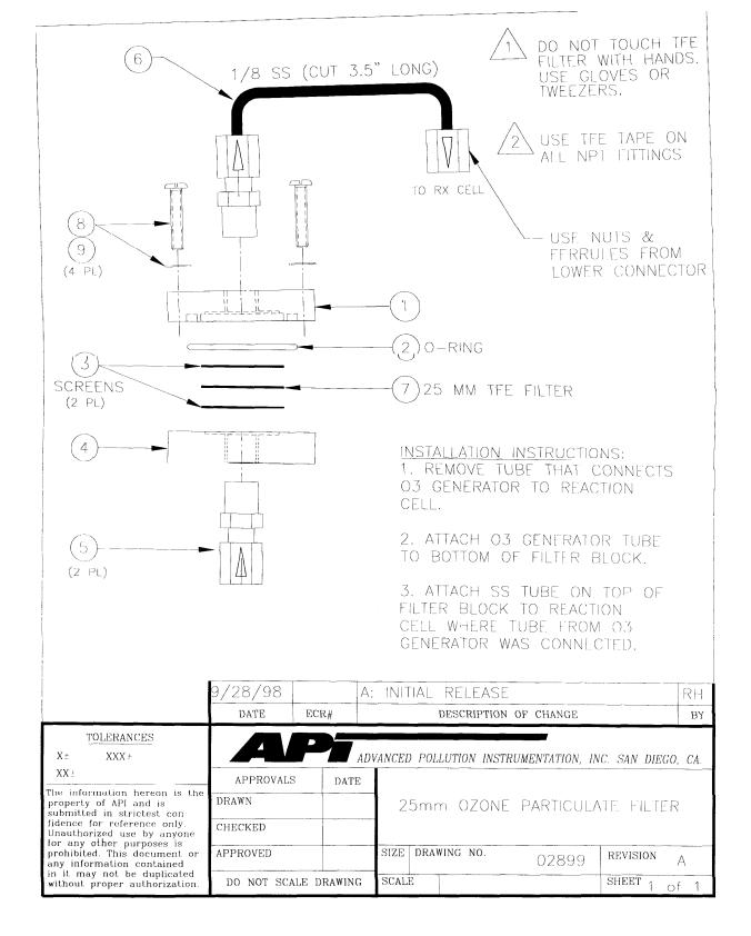
INSTALLING OZONE FILTER ON M200A/M201A/M200AH ANALYZERS Service Note-99-009 Page 2 of 3
