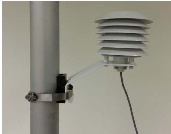
Figure 2-11. Ambient Temperature Probe Installed in Solar Shield
