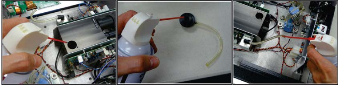
Figure 5-10. Maintenance: Final Dusting
