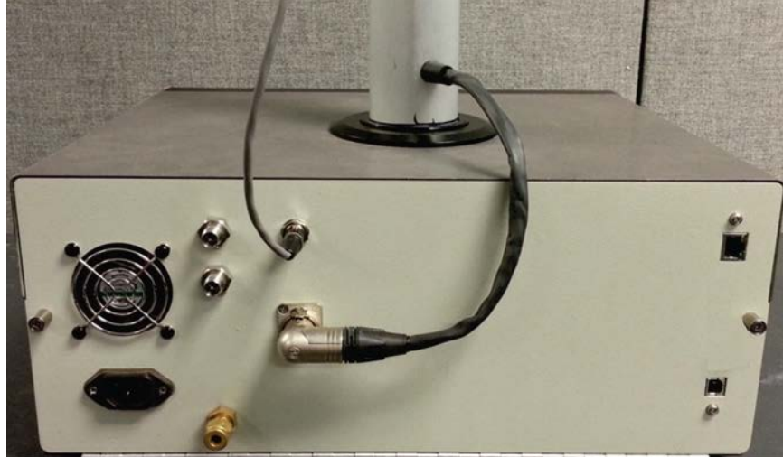
Figure 2-10. Ambient Temperature Probe and ASC Connections (T640 with 640X Option shown)
