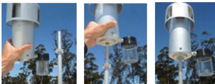
Figure 2-18. T640 Inlet and Sample Line Assembly
