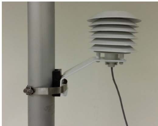
Figure 2-15. Ambient Temperature Sensor Probe Installed into Radiation Shield
