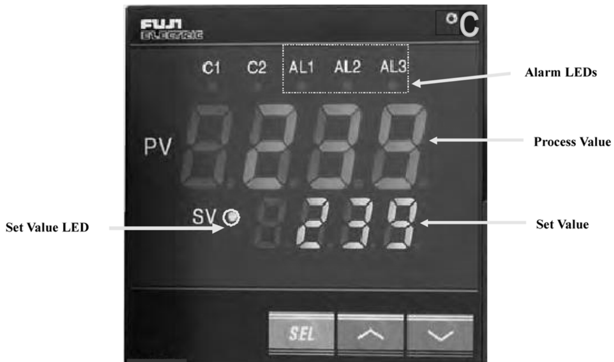
Figure 4-6. M501-TRS Temperature Controller Startup
