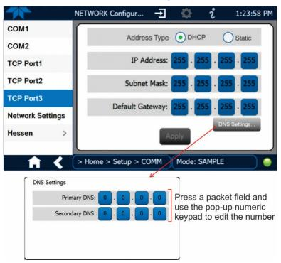
Figure 2-45. Communications Configuration, Network Settings
