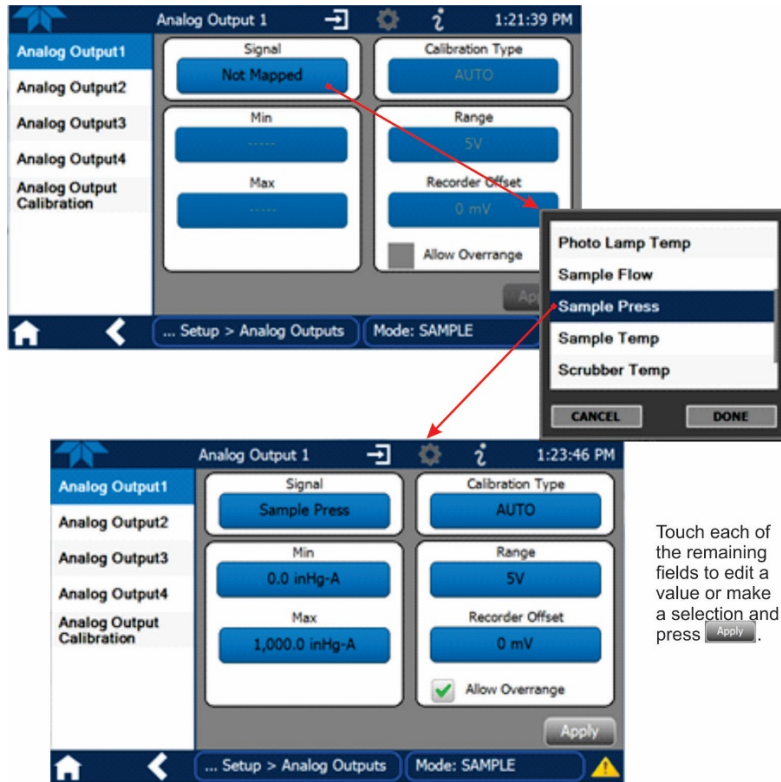
Figure 3-30. Analog Output Configuration Example
